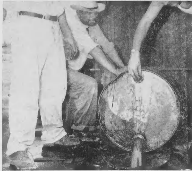
Porfilio Van der Biezen brings a drum of raw aloe juice to the factory for processing. Here it is being poured into an underground cistern for storage before it is refined.
